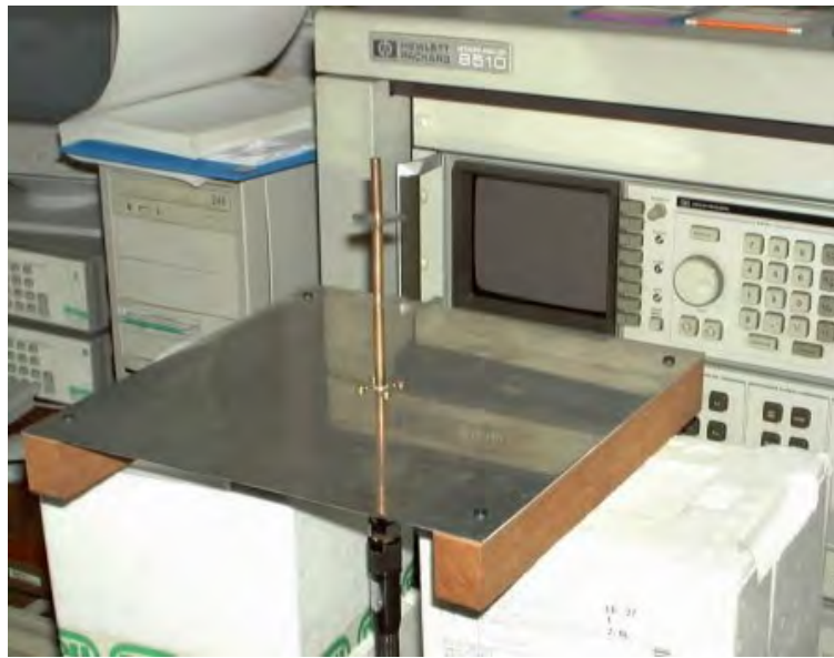
Figure 5.5 Capacitively loaded monopole on a finite square ground plane
