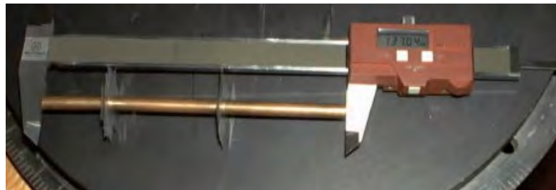
Figure 5.9 Loaded monopole of total height 137.04mm
