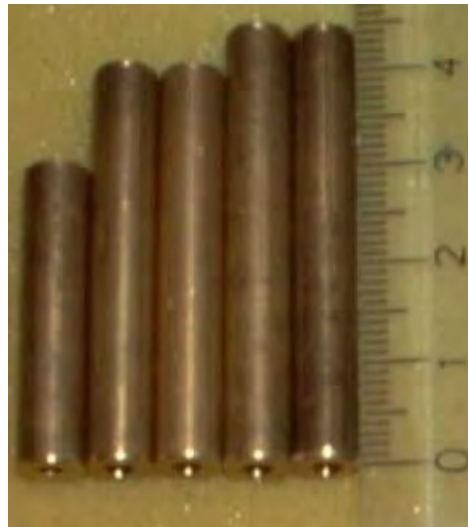
Figure 5.1 Brass rods of the monopole (The scale is in centimetres.)
