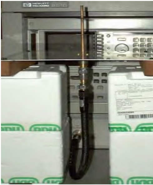
Figure 5.8 Loaded monopole and N-type connector with SMA adapter, under the ground plane
