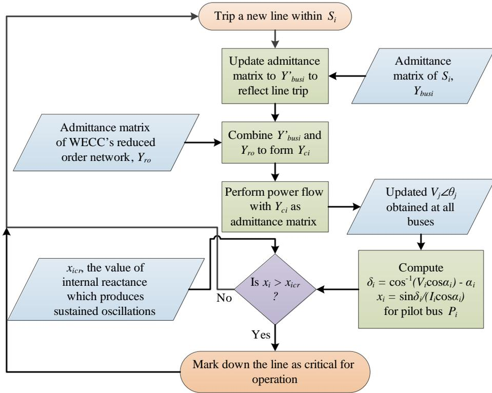
Figure 8: Algorithm for determining post-fault stability
