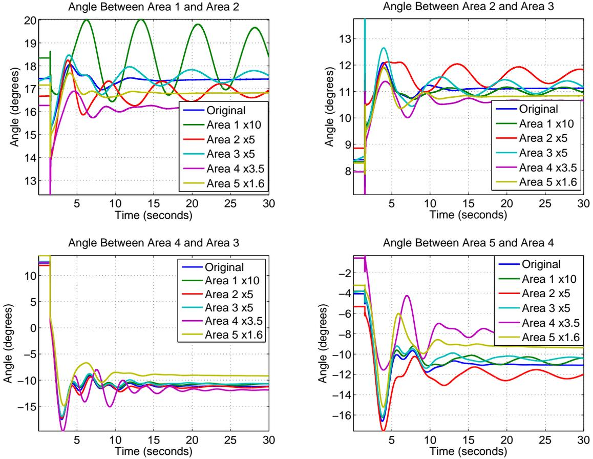
Figure 7: Contingency analysis of 5-area WECC model for local line trips
