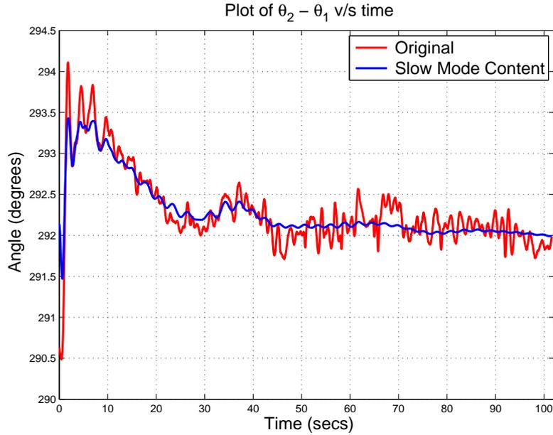
Figure 3: Slow mode component of Voltage angle difference between Station 2 and Station 1
