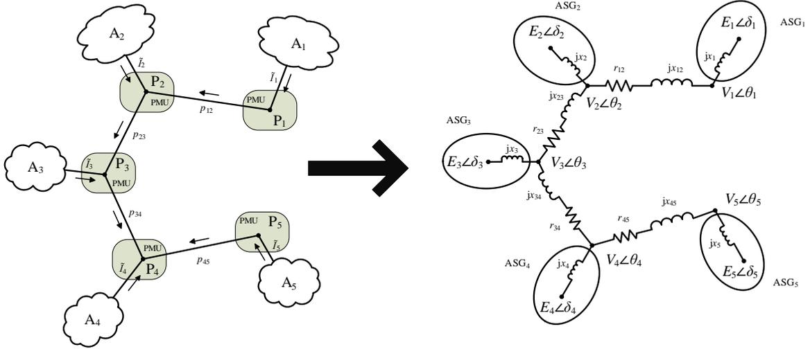
Figure 2: Electrical topology of WECC's 500kV network
