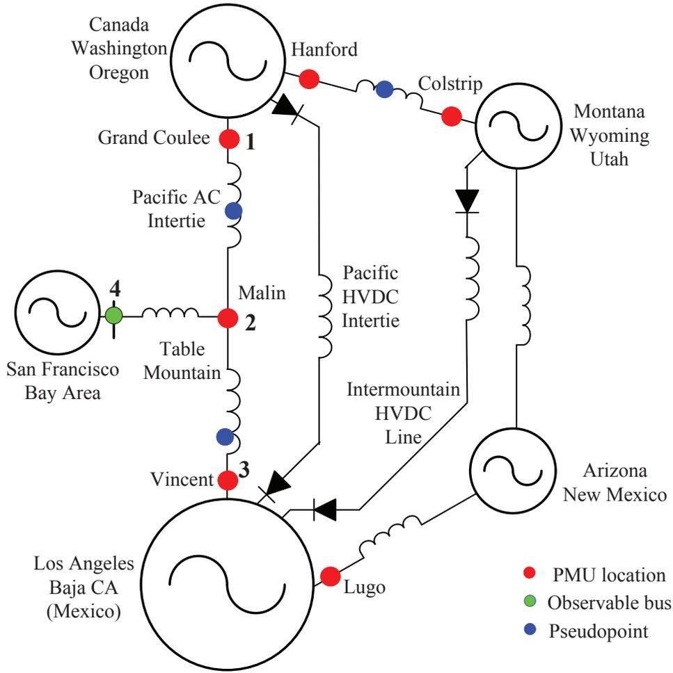
Figure 1: A 5-area dynamic equivalent model for the WECC power system
