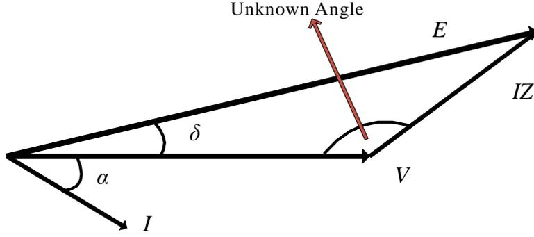
Figure 4: Phasor Diagram for the Aggregated Synchronous Generator
