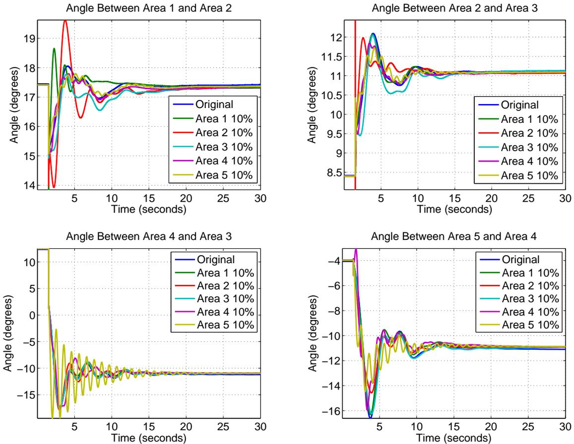
Figure 6: Contingency analysis of 5-area WECC model for loss of inertia
