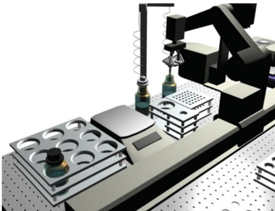
Figure 1 Model of an ORCA programmed for liquid dispensing.
