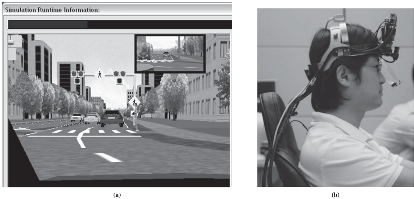
FIGURE 1 Roundabout simulation: (a) driving simulator screenshot and (b) eye tracker used in the study. (Source for 1b: Ergolab at North Carolina State University.)
