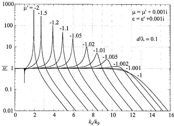
FIG. 1. Transfer function for a left-handed slab. For the perfect lens, the transfer function would be unity for all  $k_x$ . However, the deviation of either the real or imaginary part of  $\mu$  limits the range of  $k_x$ , so that the slab acts as a low-pass filter. The losses, inherent to left-handed materials, also remove the singularities that appear in the transfer function.
