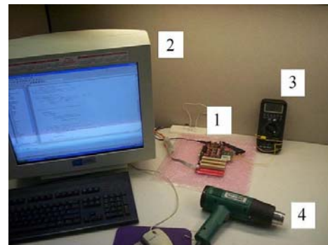
Figure 1. Experimental setup for testing page retention times.
