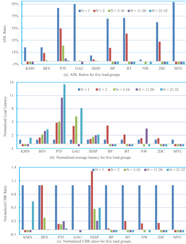
Figure 5. The effectiveness of L1D for load groups with different memory un-coalescing degrees. The loads are classified into five groups according to their memory un-coalescing degrees. The first group constitutes of the coherent loads, which have one memory access per load (i.e., the un-coalescing degree is 1). The other four groups include loads with 2, 3 to 10, 11 to 20, and 21 to 32 memory accesses per load, respectively. The negative values in the figure was used to highlight that there are no loads in this group.
