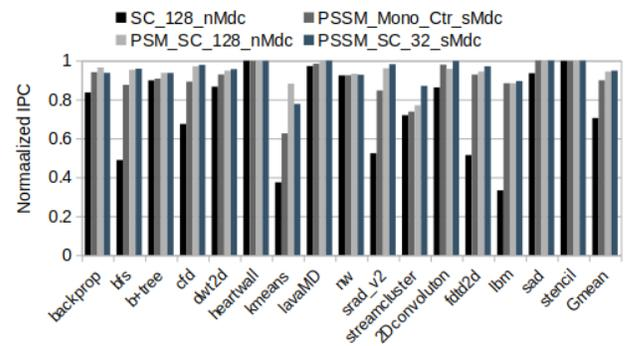
Figure 18: Normalized IPC of different GPU memory encryption schemes.
