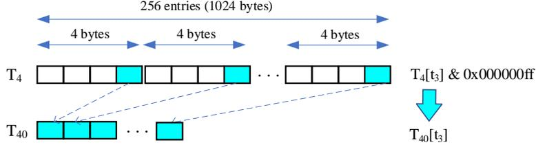
**Figure 1.** Reorganizing the table  $T_4$  in the last round of AES. The LSB of each entry is put together as  $T_{40}$ , and the next byte as  $T_{41}$ , and so on.
