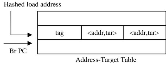
**Figure 3. An auxiliary predictor to exploit ATC.**
