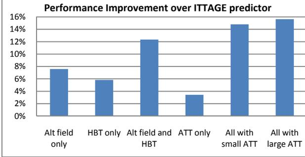
**Figure 4. The performance improvement of our proposed design over the baseline ITTAGE predictor.**
