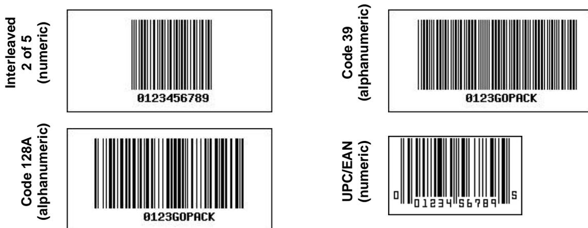
Figure 47. Bar codes used in warehousing.<sup>6</sup>
