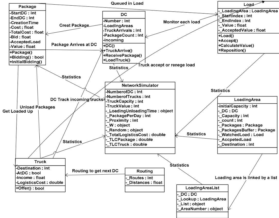
Figure 2 Object design configuration
